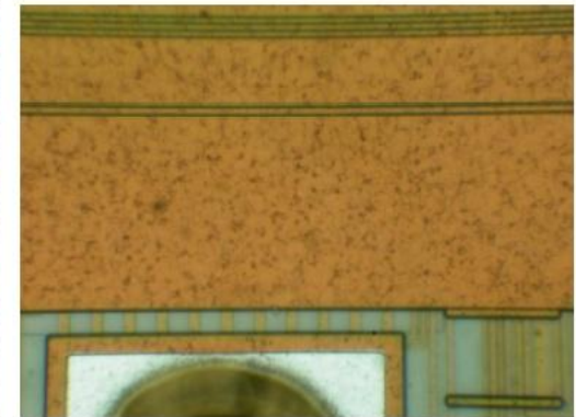
Top metal layer on microchip PIC16F877A microcontroller
